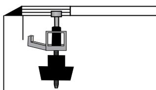
Adjust front slide-clamp to proper height.
